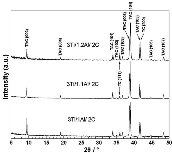
Fig. 3. XRD patterns of the samples sintered of MA powder with different Al content at 1050 °C for 5 min.
