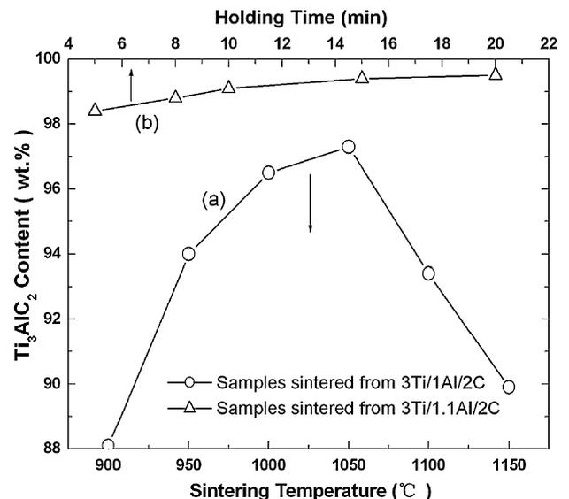
Fig. 5. (a)  $\text{Ti}_3\text{AlC}_2$  purity in the samples sintered at 900–1150 °C for 5 min. (b)  $\text{Ti}_3\text{AlC}_2$  purity in the samples sintered at 1050 °C for different holding times.
