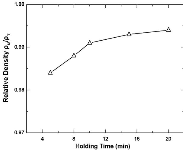
Fig. 6. The variation of relative density of the samples sintered from MA powder of 3Ti/1.1Al/2C at 1050 °C with holding time.
