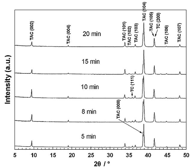
Fig. 4. XRD patterns of the samples sintered from mechanically alloyed powders of  $3\text{Ti}/1.1\text{Al}/2\text{C}$  powder mixtures at 1050 °C for different holding times.
