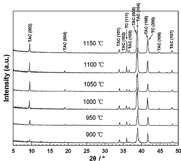
Fig. 2. XRD patterns of the samples sintered from mechanically alloyed powders of the starting composition of  $3\text{Ti}/1\text{Al}/2\text{C}$  powder mixtures at different temperatures for 5 min.
