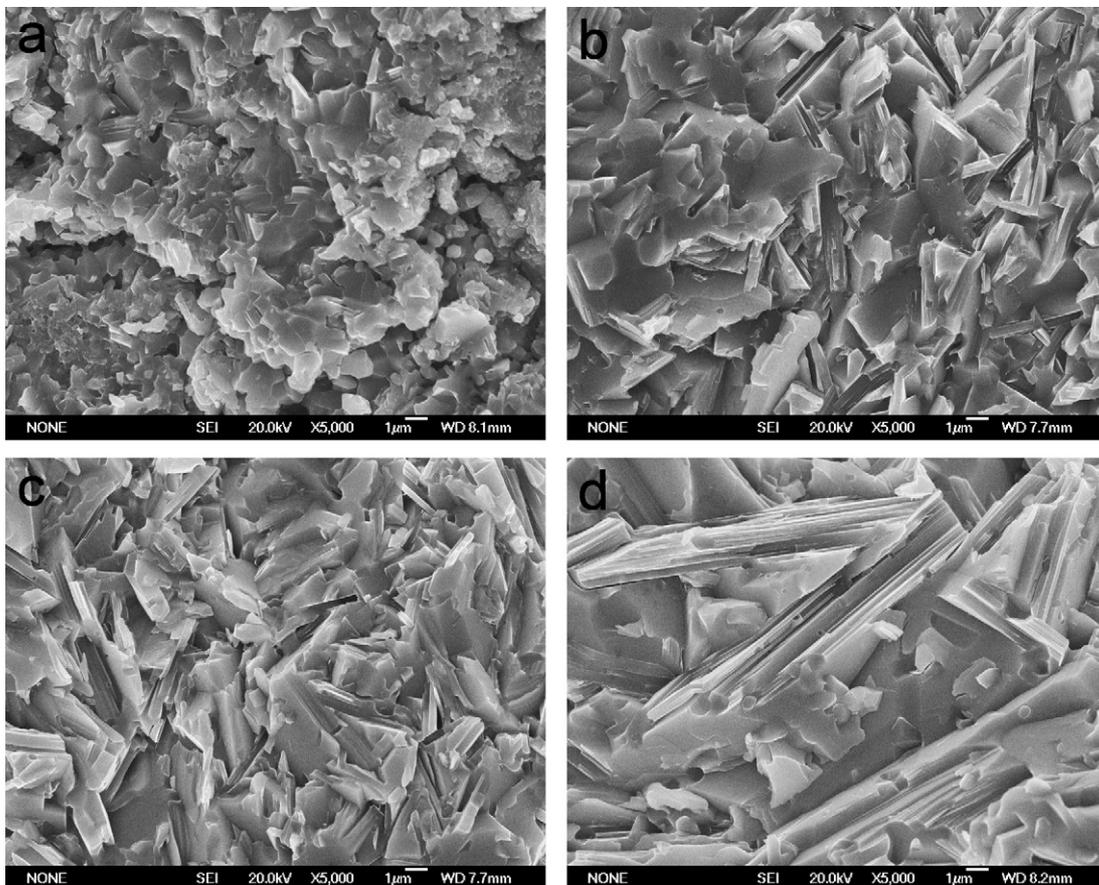
Fig. 7. SEM micrographs showing the microstructure of fracture surfaces: the samples sintered at (a) 900 °C and (b) 1050 °C for 5 min from mechanically alloyed powders of 3Ti/1Al/2C; the samples sintered at 1050 °C for (c) 5 min and (d) 20 min from mechanically alloyed powders of 3Ti/1.1Al/2C.
