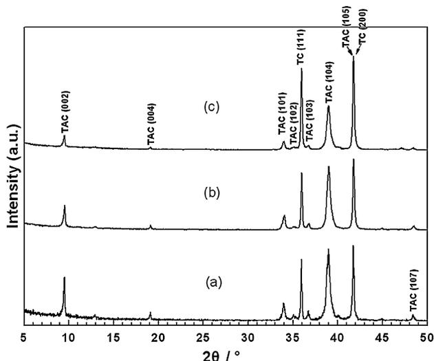
Fig. 1. XRD patterns of the powders formed by 9.5 h mechanical alloying of different starting mixtures: (a)  $3\text{Ti}/1\text{Al}/2\text{C}$ , (b)  $3\text{Ti}/1.1\text{Al}/2\text{C}$  and (c)  $3\text{Ti}/1.2\text{Al}/2\text{C}$ . TAC and TC stand for the  $\text{Ti}_3\text{AlC}_2$  and TiC, respectively.
